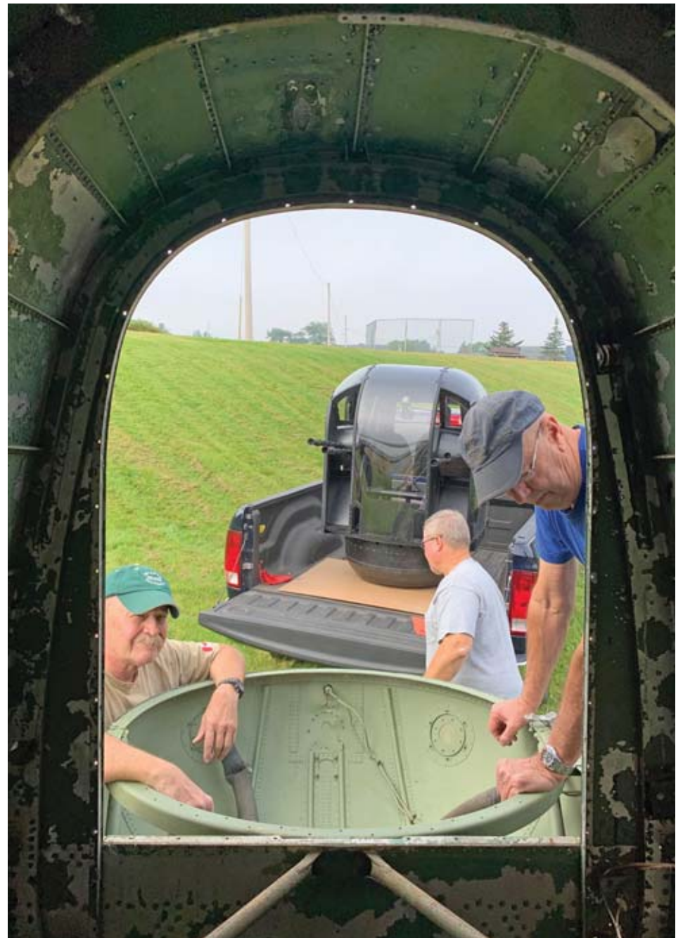
Robert Mullan, left, Marc Beaulac and Marc Allain plan the placement of the Greenwood Military Aviation's Museum's restoration Lancaster tail turret September 8.
